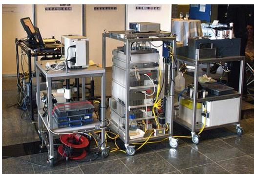
High-performance liquid chromatography (HPLC) is a chromatographic technique which separates mixtures of compounds based on their diverse chemical and physical properties, such as polarity, charge and size, using a solid phase (column) and a liquid phase. It is a method for separation using a suitable detection method (eg. UV absorption or mass spectrometry) for the identification and quantification of substances.
