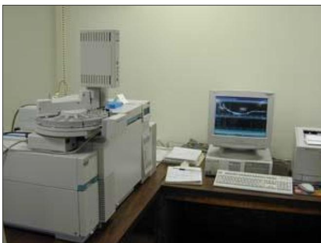
Gas chromatography (GC) analysis is a widespread methodology employed to confirm the presence of chemical substances. This makes it attractive for drug and drug contaminant testing. GC analysis separates the components of a drug sample and a spectral output is generated.
